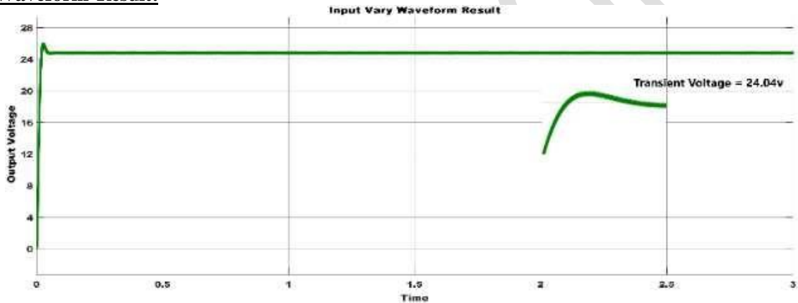
Fig.6.18. 8V Input vary for boost converter performance using FLC.
